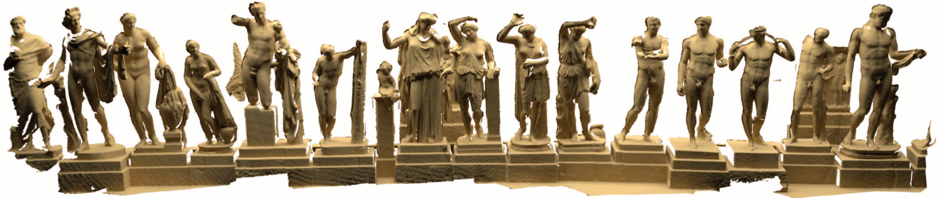
Figure 1: Example output from our reconstruction system without any geometry post-processing. Scene is about 20m wide and 4m high and captured online in less than 5 minutes with live feedback of the reconstruction.
