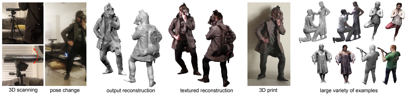
Figure 1: With our system, users can scan themselves with a single 3D sensor by rotating the same pose for a few different views (typically eight, \sim 45 degrees apart) to cover the full body. Our method robustly registers and merges different scans into a watertight surface with consistent texture in spite of shape changes during repositioning, and lighting differences between the scans. These surfaces are suitable for applications such as online avatars or 3D printing (the miniature shown here was printed using a ZPrinter 650.)
