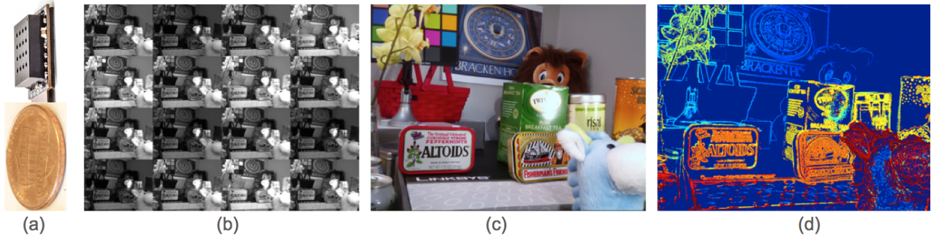
Figure 1: From left to right - (a) The PiCam Camera Array Module (b) Raw 4 \times 4 array images each 1000 \times 750 pixels (c) Parallax corrected and superresolved high resolution 8MP Image; (d) A high resolution filtered 8MP depth map
