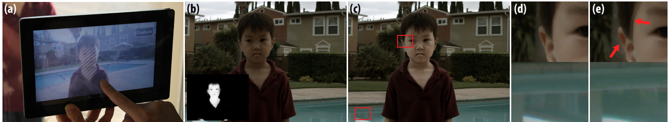
Figure 1: Viewfinder editing and appearance-based metering. (a) In the proposed system, the user interacts with the camera viewfinder as if it were a live canvas, by making sparse strokes to select regions and to specify edits. The edits propagate spatiotemporally as the camera and the scene objects move, and the edits are applied in the subsequent frames of the viewfinder, which are tonemapped HDR images, to provide WYSIWYG experience. (b) After making a local tonal edit, the user presses the shutter to trigger a high-resolution capture. Here we show the resulting tonemapped HDR composite without any edits applied, for reference. The edit mask computed from the user strokes is shown in the inset. (c) The result with edits applied is shown. This approximately corresponds to what the user sees on the screen just as he presses the shutter. Our appearance-based metering acquired an exposure stack at (0.645 ms, 5.555 ms, 11.101 ms) by optimizing the quality of the final result based on the user's global and local edits. (d) The regions indicated in (c), magnified. (e) We captured another stack with a histogram-based HDR metering at (0.579 ms, 9.958 ms, 23.879 ms) and applied the same post-processing pipeline. As the standard HDR metering considers equally all the pixels in the scene, it allocates too much effort to capture the dark areas that were not as important to the user, leading to a longer capture times that invite ghosting (top) and higher noise in mid-tones (bottom).
